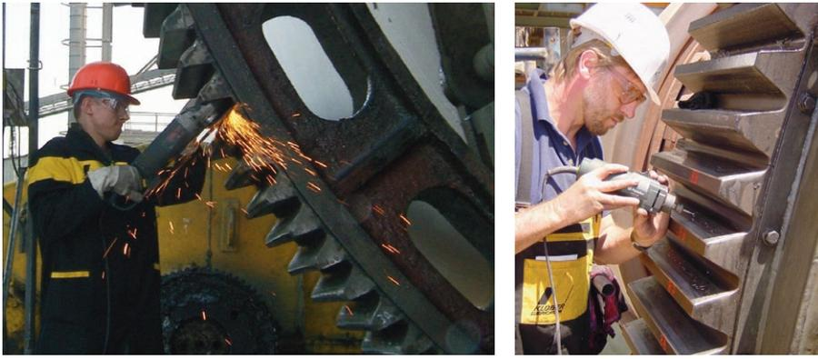
Figure 5. Mechanical treatment of tooth flanks and repair lubrication are services provided by experienced tribology specialists.
